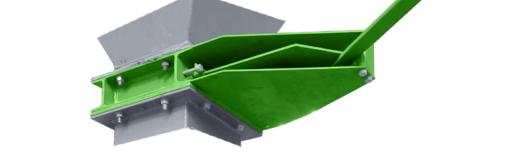
The slide gate SPA is designed for closing the hoppers and storage bunkers with loose and non-adhesive pulverized materials. They are applied in places accessible to manual control by the handwheel. The slide gate is made of rolled profiles with plate of 6 mm thick sheet.
